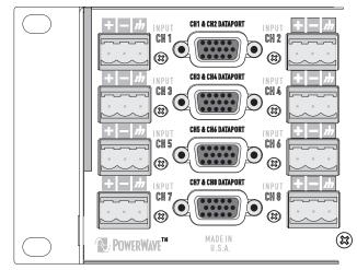
A single DataPort is assigned to each channel pair. Each DataPort is marked with the channel numbers served by that DataPort. Note, above, that each DataPort is clearly labeled and is located between its respective channel's terminal block connectors.
